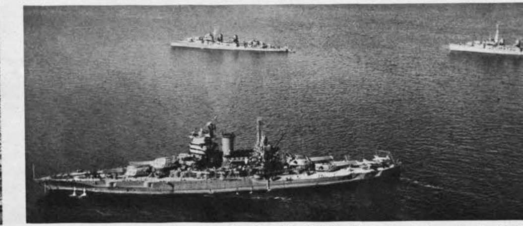
New Mexico Class somewhat resembles the older British ships. Age is shown by the lack of streamlining. Chief distinctions are a raked clipper bow and short masts, bridge and stack.
